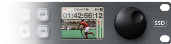
The LCD on HyperDeck Studio models displays embedded SDI timecode when the option to "Use SDI video input timecode when recording" is switched on.
