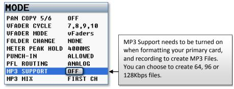
To record MP3 files you will need to first format your primary card with the **MP3 SUPPORT** turned on to create an MP3 folder on the primary card. Formatting the card will create a large (700Mbyte) loop onto the PRIMARY card. This loop will hold up to 24 hours of MP3 audio (at 64kbps).
