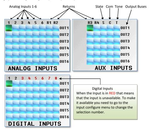
To move between the matrixes, press the BUS key.
