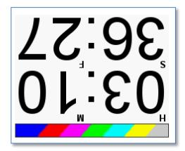
Pressing the **TC** key once brings you to, an inverted visual timecode slate. Pressing the **MENU** knob will freeze the display and cause a 1-frame long beep tone in the audio on any bus that is selected for tone output.
