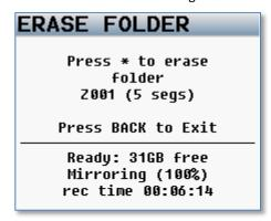
WARNING: If you have mirrored a folder and need to erase it to make room for more recording files on the primary card, REMOVE the MIRROR card before doing the erase. If you don't, the folder will be ERASED FROM BOTH CARDS!
