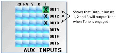
**NOTE**: Only the busses with tone routed to it will output the slate tone when the Visual Timecode Slate tone is activated
