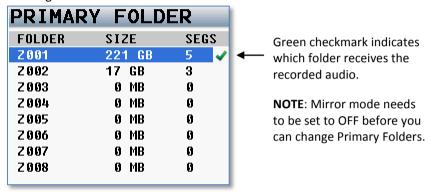
All recorded files are directed to individual folders. This allows you to choose which folder is being used for recording. The folder can be renamed to help identify its contents. To name your folder hit the back button and in the **PRIMRY CF** menu then scroll down to the **Edit Current Folder Name** then press **MENU** to change the name of the folder.
