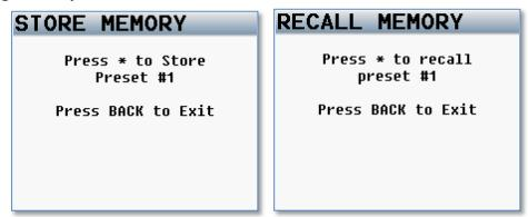
From this menu, Nomad can save and recall three full recorder setups for different work scenarios. All user set parameters are saved and can be recalled as needed.
