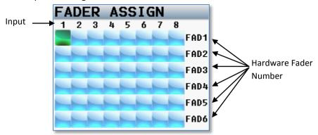
Because Nomad is a digital mixer, no actual audio is going through the Nomad Fader controls allowing for complete flexibility for the mixing hardware faders. Any one of the analog inputs 1-8, digital inputs 1-8, analog trim controls or ZaxNet trim can be routed to any hardware fader.
