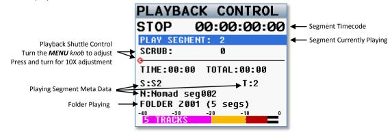
**NOTE:** While in this menu, the **STOP** key and **PLAY** key function immediately, even if the **Transport Keys** are set to shifted mode.
