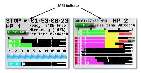
If MP3 SUPPORT is on in the Mode menu all files will be "marked" by default. If you don't want to create an MP3 of a particular file you can toggle it off by pressing the A-MIX key before or while recording.
