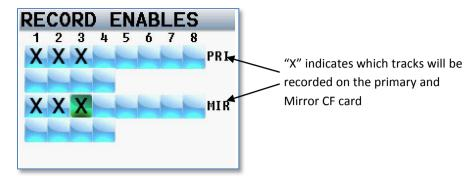
NOTE: If sample-rate is set to 88.2 kHz or 96 kHz, only eight Primary and Mirror tracks can be selected and recorded
