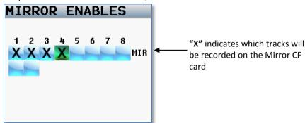
**SHORTCUT:** It is not necessary to remove record enable cross points from the Mirror Matrix. If a Primary card track doesn't have anything routed to it; it will NOT be recorded and therefore NOT written to the Mirror card. This allows you to leave all of the Mirror tracks enabled. This makes it unnecessary to change the tracks being mirrored every time you change a tracks record enable state.
