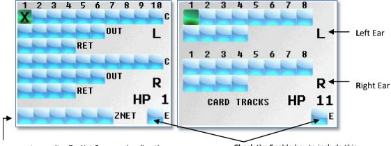
**Allows** you to monitor ZaxNet Frequencies directly NOTE: You can only choose one ZaxNet Frequency at a time. (click **IFB RX Channel Setup page**)
