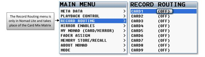
The record routing in Nomad Lite is slightly different from the card routing in Nomad 10 or 12. Nomad Lite doesn't have a record enable matrix or a card routing matrix. With Nomad Lite, you can route all your inputs and all your record busses to any one of the 10 record tracks.
