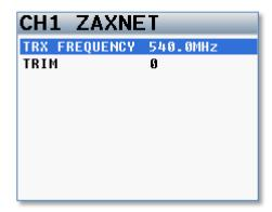
When you are in this menu, if you press a multi-function channel key you will change which ZaxNet transmitter's parameters you adjust.
