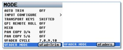
When the virtual fader is active the bottom meter on the **ENG Meter Screen** will display what you will be controlling. Either fader only or fader and trim for an input channel.
