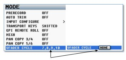
Shows which inputs will be available when the Virtual Fader is activated
