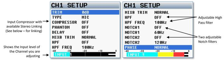
While in this page, pressing any of the multi-function keys will jump to the **Setup page** of the corresponding input channels one through ten.
